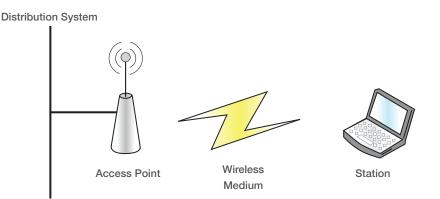
WLANs use the RF spectrum to carry information just as smartphones and two-way radios do. Just like these other technologies, WLANs operate on either of two frequency ranges, the 2.4 GHz and 5 GHz bands. Each band has a number of channels: 2.4 GHz has 14 channels while 5 GHz has 24 channels. (In the US, the FCC limits the use of some of these channels.) These channels provide the physical media to carry the information, just as an Ethernet cable or two-way radio channel does.
