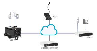
A WAIS can include any number of operators and communications end points (radios, phones, etc.) interfaced via ACU-Ms and other ACU devices, all networked together.
